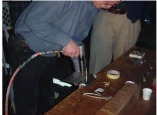
Bruce noted that if you anneal the rivets first, then they will be easier to drive with less deformation of the metal being riveted. He noted that old, hard rivets can be like nails! Heat the rivets up to 750 to 790 degrees Fahrenheit for 15 minutes, then quench them in ice cold water. They will start to get hard again in 24 hours or so. Keep the rivets in a refrigerator or freezer to keep them soft longer.
