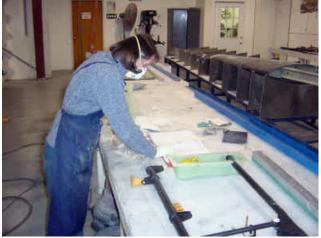
Sara is assembling the aileron control mechanism. The green tray contains the control stick rod and the aileron bell crank (yellow piece). A seal will go in the middle of the tray and a lid will be put on. One side of the seal will be open to the exterior to allow the control rod to go out to the wing, while the other side will have cabin pressure on it. Next to the green tray is the elevator crossover tube that will be mounted behind the cabin.
