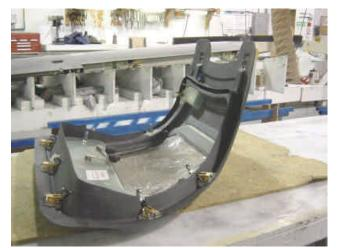
The Fastbuild kit provides the door and the frame together. There are two door handles -- one operates the bottom latches and the other operates the side latches. Eight latches and two sturdy hinges are needed to withstand the roughly 5000 pounds of force from the cabin pressure.
