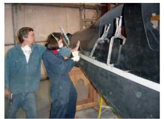
The top of the fuselage has been set in place on the bottom. Sara is installing Clecos to temporarily hold the top and bottom together.
