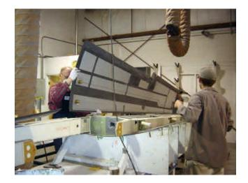
The wing is upside down and the bottom skin is being set in place over the speed brake assembly so that the reinforcing pocket can bond to the wing skin. The brass fittings near Harvard's hand are fuel drains.
