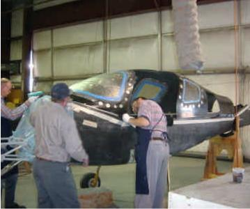
The fuselage top with the windows newly installed is placed on the bottom to prevent any mismatch between the top and bottom as the window glue sets up. Note the bolts with large washers around each window.
