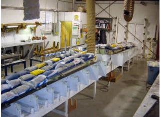
After structural glue is applied to the wing assemblies and the wing skins, long straight bars and bags of lead shot are piled on the wings to get a good joint. Each bag weighs about 25 pounds. A couple thousand pounds are put on each wing!
