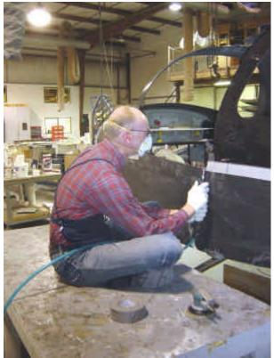
The doorframe has been fitted, marked, and then removed again, and Harvard is trimming up the fuselage to accommodate the doorframe.
