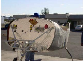
The fuselage has arrived back from the shop where some of the fittings were installed on the firewall.
