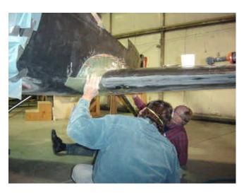
The wings are bolted onto the fuselage and the wing fairings are fitted between the fuselage and the inner edge of the wing. The fairing rib, temporarily attached to the wing, holds the fairing in the correct position on the wing, while clecos are used to attach the fairings to the fuselage. Kerry, our technician, and Harvard check the fit of the lower fairing piece.
