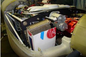
Joe (mostly) and Steve Senatori built this plans-built Sierra helicopter, powered by a Lycoming 320. Joe did all the welding on the tubular steel frame.
